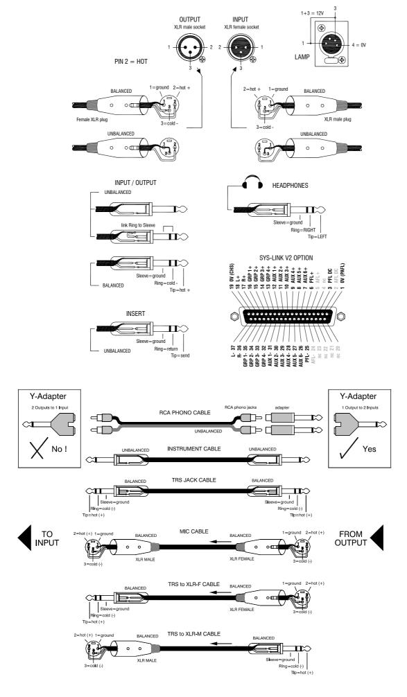
The GL2400 uses professional grade 3 pin XLR and 1/4" TRS (3 pole) jack sockets. To ensure best performance, we recommend that you use high quality audio cables and connectors, and take time to check for reliable and accurate cable assembly. It is well known that most audio system problems are due to faulty or sub standard interconnecting leads. The following plugs may be used to connect audio to the console:
