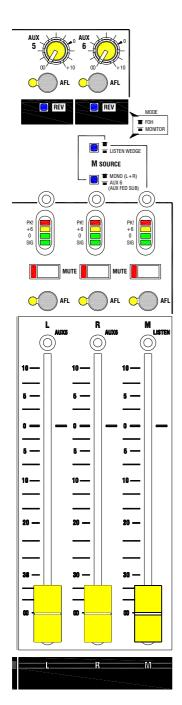
**AUX 5 and 6 Masters** These function in the same way as described for auxes 1 to 4. In monitor mode, the recessed REV switch reverses the AUX5 master with L, and AUX6 with R. Here the aux signals are presented to the L and R XLR outputs complete with their inserts. The LR mix swaps on to the Aux TRS jack outputs. Note that the LR mix always feeds the matrix and 2-track regardless of mode selected.
