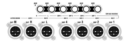
**GROUP, L, R, M OUT** The main console mix outputs are on electronically balanced XLR. These produce the professional standard +4dBu when the meters read '0', and provide up to a maximum +25dBu. The L and R outputs typically feed the house PA system in live sound mixing, or a 2-track recorder in studio mixing. In monitor mode, these outputs reverse with the Aux TRS jack connections.
