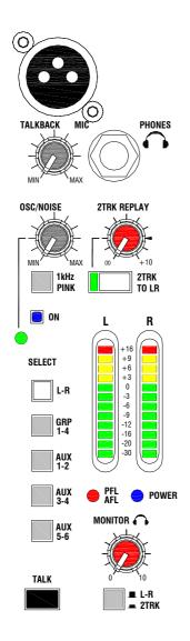
**Console Monitor** Comprehensive engineer's headphones and local monitoring is provided. Select either LR or 2-track return as the default source using the L-R / 2TRK switch. Pressing PFL or AFL elsewhere on the console automatically overrides the current monitor source with the signal from the channel or master selection. The red PFL/AFL active indicator illuminates and the console meters display the active signal.
