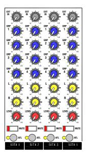
**Applications for the Matrix** The matrix is a 'mixer within a mixer', a versatile toolbox of outputs you can use to satisfy a host of applications. Each of the 4 outputs is mixed from any combination of the groups, L, R and an external input as dialled up on the 7 source rotaries (hence a '7x4' matrix). Its master level can be adjusted independently. Using combinations of the outputs you can create mono, stereo or multiple output mixes. Some applications include:
