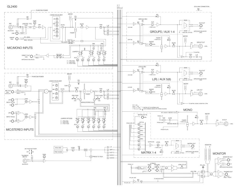
The GL2400 has a versatile architecture which should satisfy most applications you may encounter without modification. However, the following internal options provide alternative settings for those applications that may demand them. Access is required to the internal assemblies. For user convenience, pluggable jumper links are used in most places.
